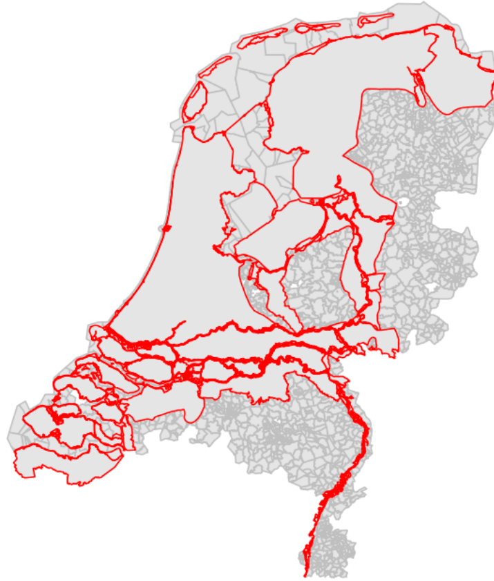
Fig. 2. Flood risk zones in the Netherlands considered in the stress test. This figure shows the areas of the Netherlands which are vulnerable to two main types of flood. The first type would impact unprotected areas (in red), the second flood type would impact protected areas (in light gray) that are mainly located in the western half of the Netherlands.
